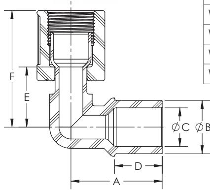
**Weld Elbow Connector (TightFLARE™)**
