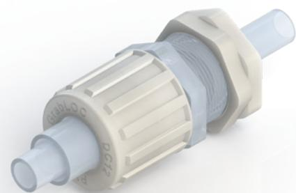
**MCDC series** fittings are used on a box or cabinet that have a female NPT. The primary tubing passes through the fitting body with a simple push-on secondary tubing terminating the tube connection. There is no flaring required of the secondary tube.
