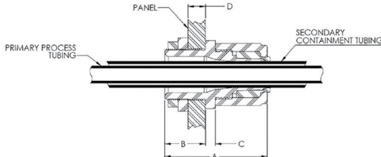
**MCBP series** fittings are used on a box or cabinet that have a female NPT. The primary and secondary tubing pass through the fitting body. This allows chemistry to flow back to the supply source if the primary tube leaks.
