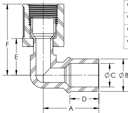
**Weld Elbow Connector (TightFLARE™)
