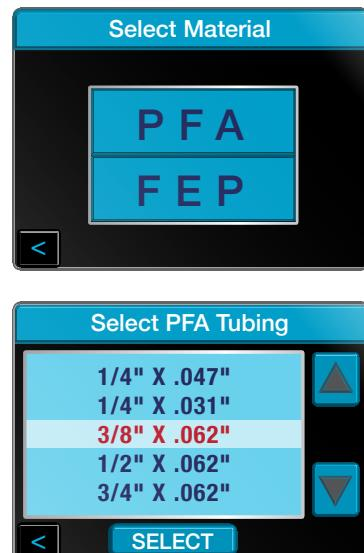
Select material and tube size and the controller will automatically set the required heat temperature, heat time and cure time. Custom settings can easily be created and saved.
