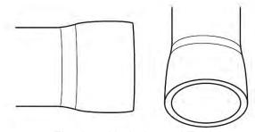
Fig. 15. Underheated Tubing
