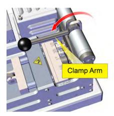
Fig. 11. Clamp Arm fully retracted
