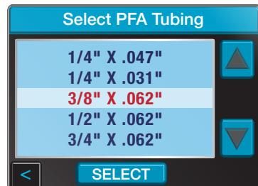
Select tube size and the controller will automatically set the required heat temperature, heat time and cure time.
