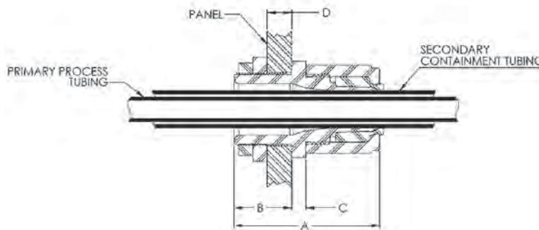
**MCBP series** fittings are used on a box or cabinet that have a female NPT. The primary and secondary tubing pass through the fitting body. This allows chemistry to flow back to the supply source if the primary tube leaks.
