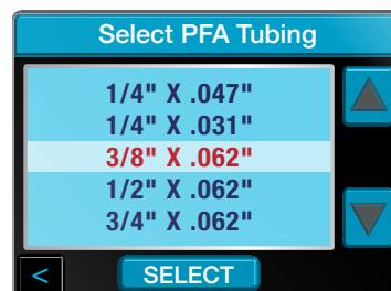
Select material and tube size and the controller will automatically set the required heat temperature, heat time and cure time. Custom settings can easily be created and saved.
