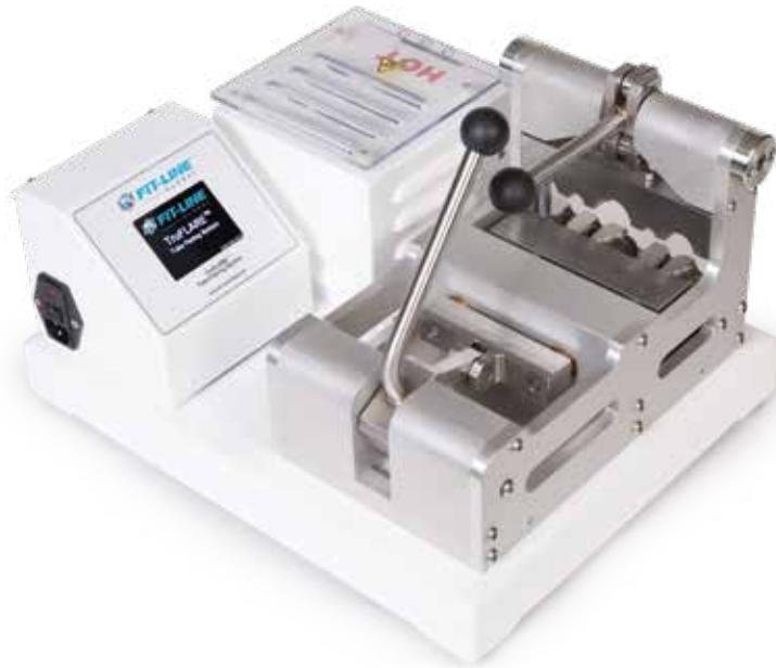
Uniquely engineered, semi-automated bench top flaring system. Creates a standard tube flare end by pressure forming and rapidly cooling the flare form. The bench top TruFLARE™ system is ideal for production flaring. It assures precise, concentric, repeatable tube flare connections. This requires no immediate assembly, which is often the case with other rudimentary hot flaring systems.
