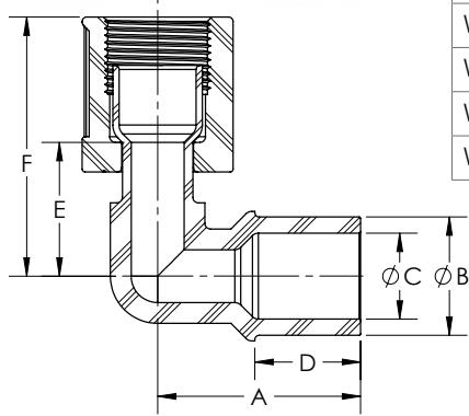
**Weld Elbow Connector (TightFLARE™)**
