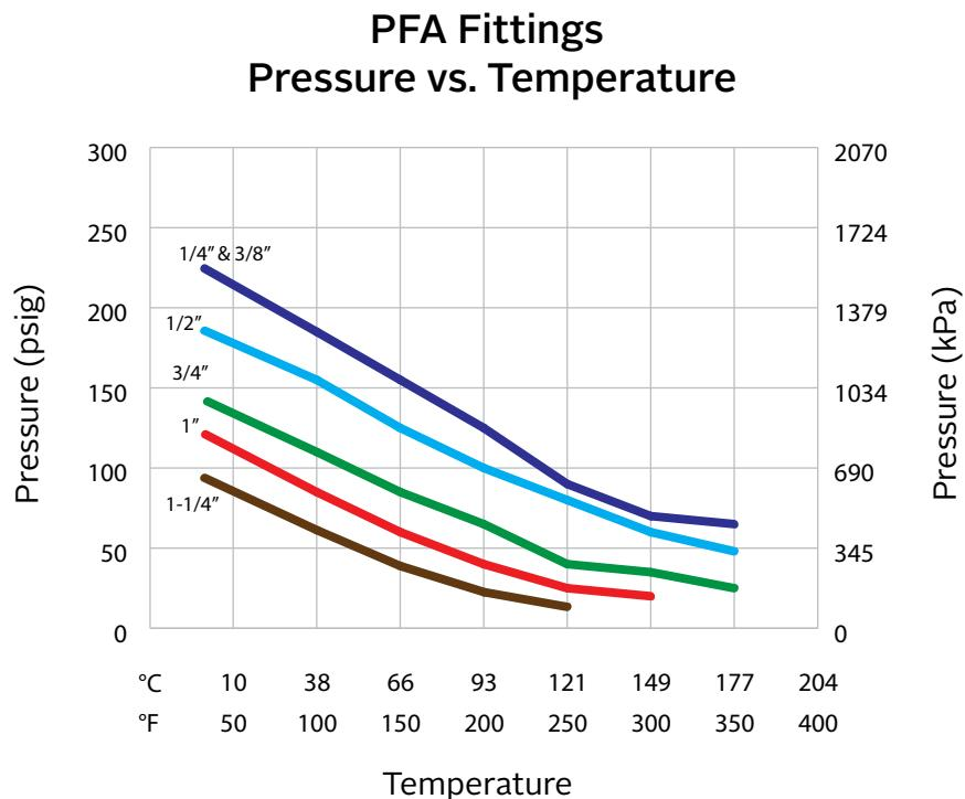
Pressure ratings for 1/4" flares are based on 0.047" wall tubing; 3/8", 1/2", 3/4" and 1" flares are based on 0.062" wall tubing and 1-1/4" flares are based on 0.075" wall tubing.
