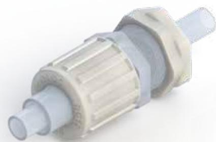
**MCDC series** fittings are used on a box or cabinet that have a female NPT. The primary tubing passes through the fitting body with a simple push-on secondary tubing terminating the tube connection. There is no flaring required of the secondary tube.
