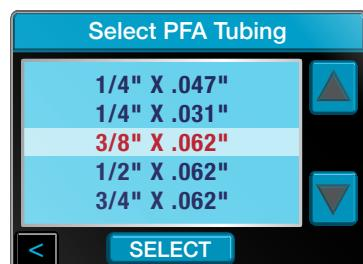
Select tube size and the controller will automatically set the required heat temperature, heat time and cure time.
